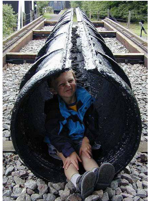
A section of pipe from Brunel's atmospheric railway at Didcot Railway Centre - a four-year-old child shows the scale © William M Connolley, Wikimedia Commons (CCL)
